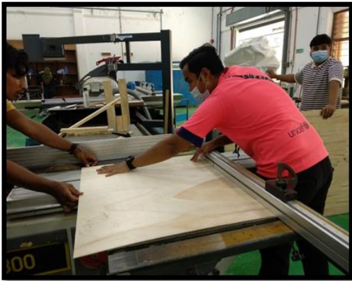
Plywood cutting process using table saw
