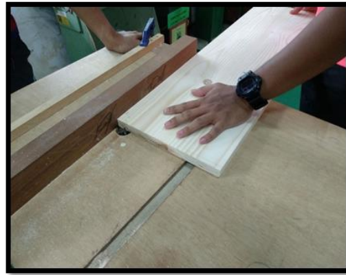
Groove making process using trimmer
