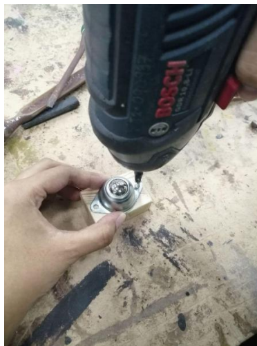
Ball bearing installation
