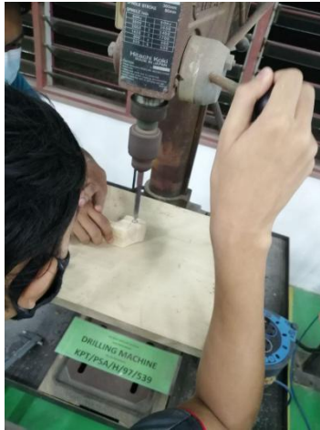
Process to make a hole using drilling machine
