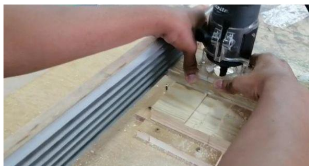
Process to make a curve shape using trimmer
