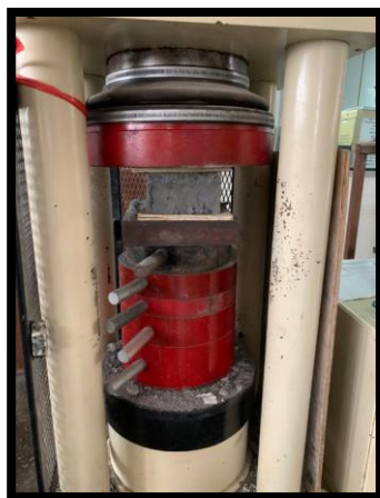
Figure 4: Testing of compressive strength and water absorption tested on HDPE-cement brick samples
