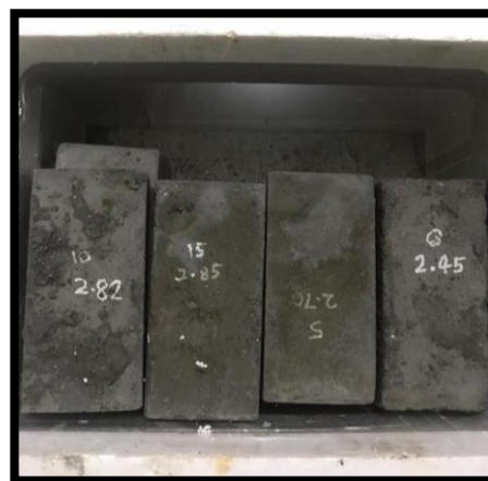
Figure 4: Testing of compressive strength and water absorption tested on HDPE-cement brick samples
