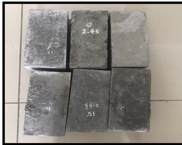
Figure 3: HDPE-cement brick sample that has been replaced with plastic waste with replacement
