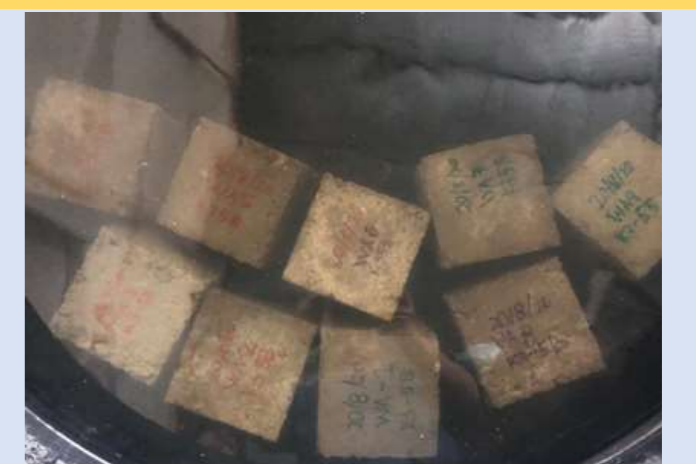
6. Curing the concrete sample in tank.
