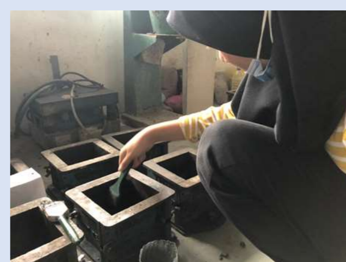
3. Oil the mould before put concrete into it.
