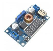
To manage our power and to power the charged electronics we need a regulator to manage the power so electricity overflow can be avoided. In our project, we decided to use a DC-DC buck converter that equipped with a TFT display and a USB port to charge the electronics. It can be found at an electronic store everywhere and it is easily maintained when broken. A new one is also affordable and selling at a quite cheap price so maintenance is a small matter.
