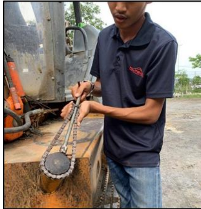
Figure 4.4.2 - Combination of chain and modified socket can open any object with cylindrical shape
