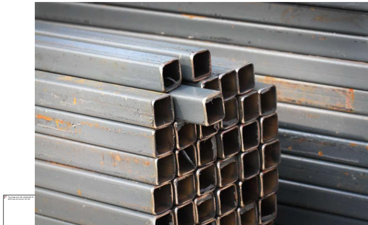
Rajah 3.4.12 Mild Steel Hollow Bar
