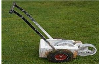
Figure 2.1 Manual Line Marking
