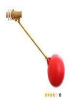
It consists of a valve connected to a hollow sealed float by means of a lever, mounted near the top of the tank. When the water level rises, the float will rise and the valve will shut off the water flow.
