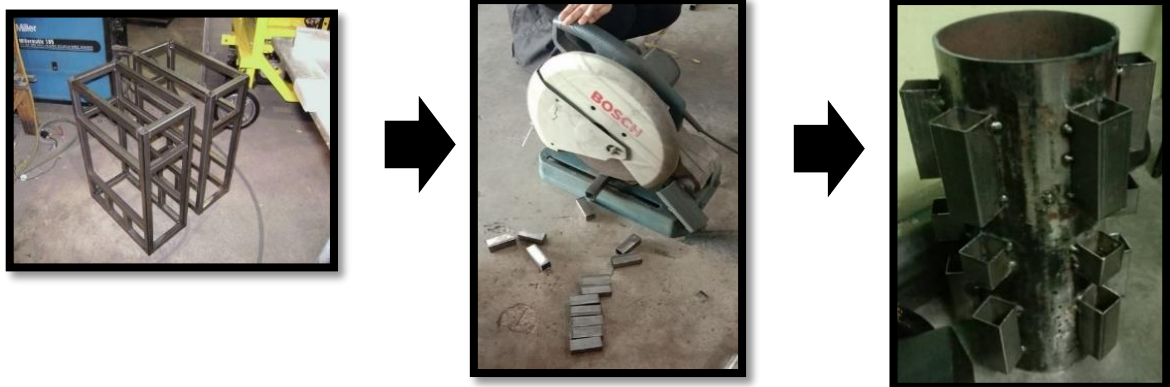
Rajah 3.4: Mengimpal rangka tong dan memotong besi Hollow
