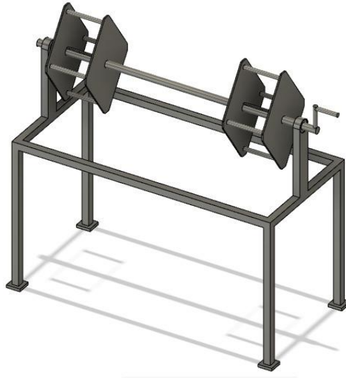
Figure 2.3 Squid Jigging Machine
