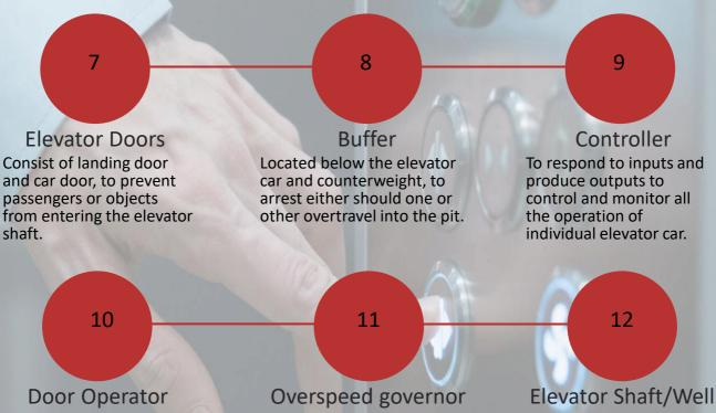
Located above the lift doors, to open and close the landing door and car door in a safe and swift manner.
