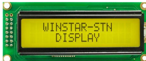
Rajah 2.3.5 : Alphanumeric LCD, 16 X 2
