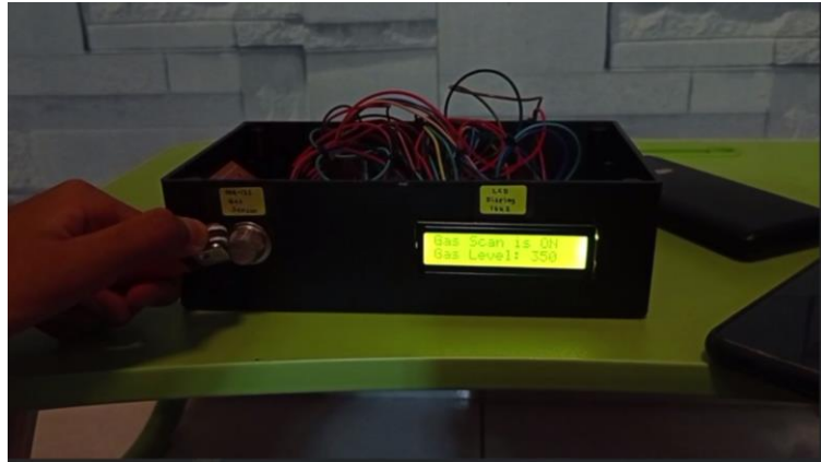
Figure 4.4: LCD display when gas is detected
