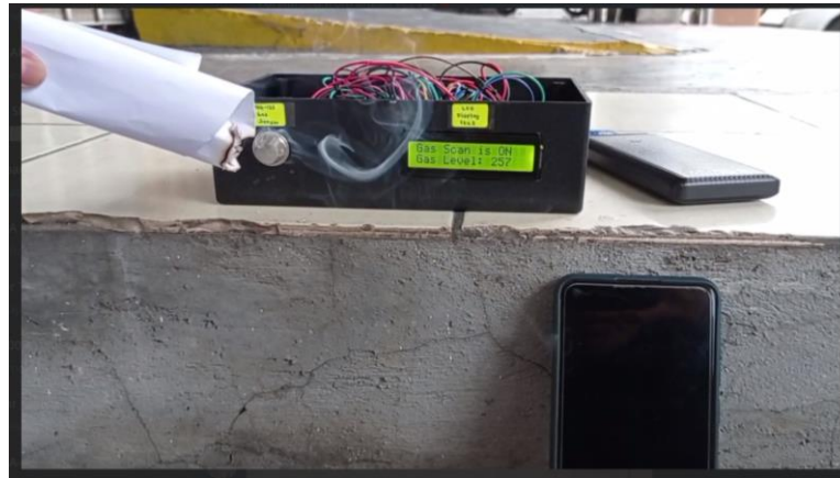
Figure 4.7: LCD display when smoke is detected
