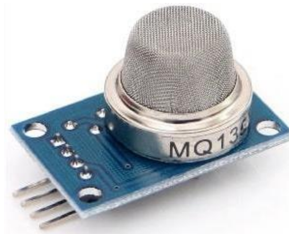
Figure 3. 6: MQ-135 Gas Sensor
