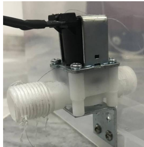
Figure 4.4: View of Solenoid Valve (Outlet)
