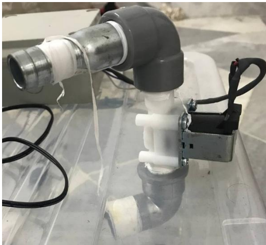
Figure 4.3: View of Solenoid Valve (Inlet)
