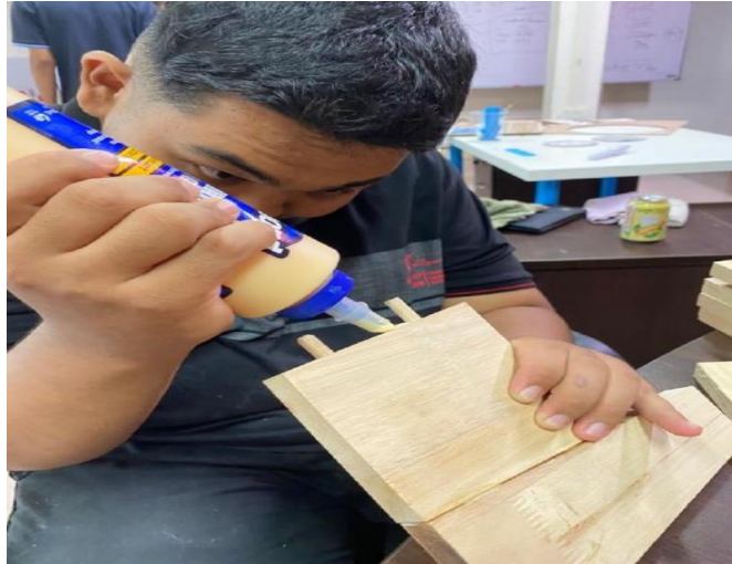
Image 3.5 (c) Showing attach dowel to table leg using wood glue.
