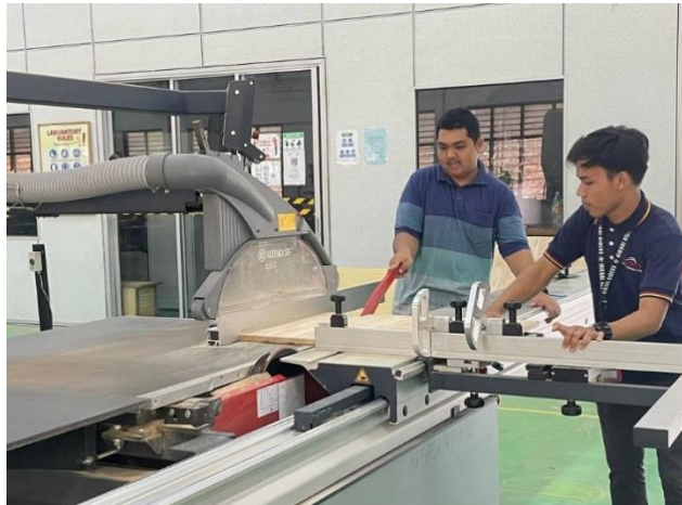
Image 3.5 (a) Showing cut a Rubberwood using Sliding Table Saw at polytechnic.
