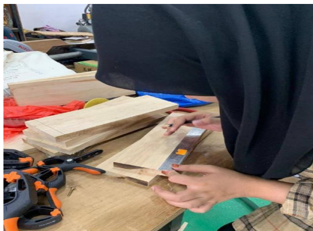
Image 3.5 (b) Showing make a measurement to make a Finger Joint.
