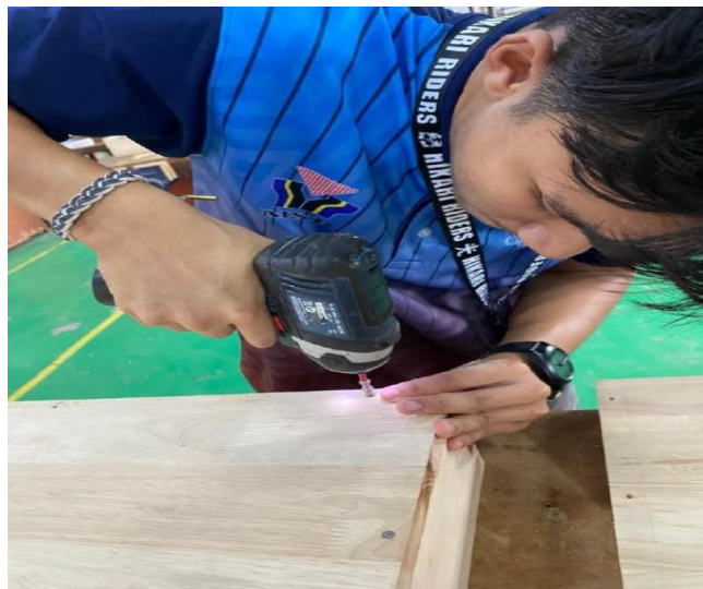
Image 3.5 (f) Showing installed dowels at table leg.
