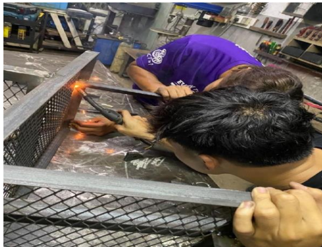
Image 3.5 (k) Showing welding a brackets.
