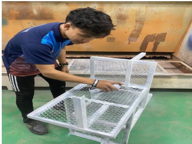
Image 3.5 (m) Showing coating the structure.
