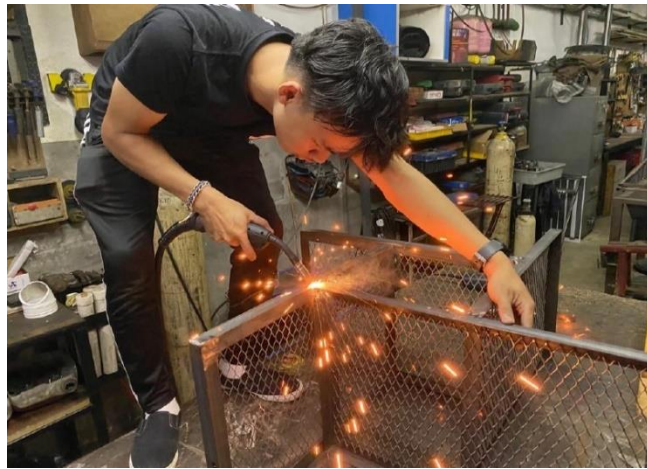
Image 3.5 (j) Showing welding expended metal.
