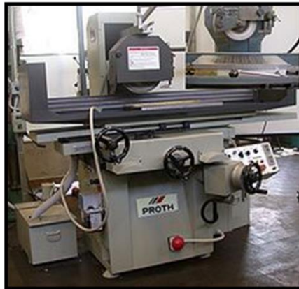
Rajah 3.7 (iii) Surface Grinding
