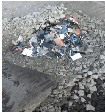
Figure 3.3.1b E-Waste mixture with concrete
