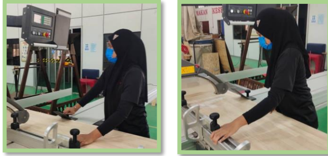
Figure 3.4: Cut the Rubberwood by using Table Saw
