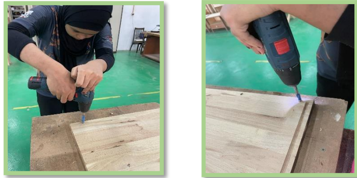
Figure 3.6: Making holes for wood dowels.
