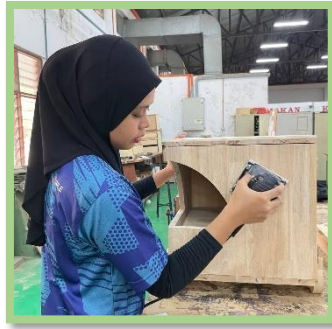
Figure 3.8: Sanding cabinet to get smooth surfaces.
