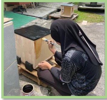
Figure 3.10: Applied shellac to all cabinet surfaces and drawers.
