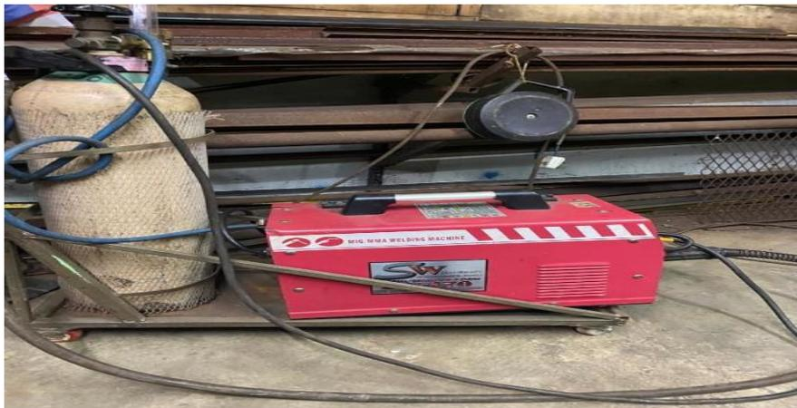
**Gambar rajah 3.6: Mesin kimpalan**
