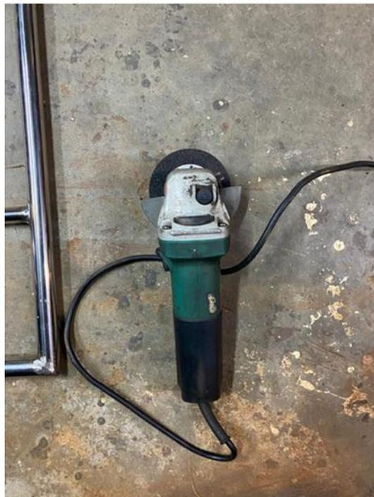
**Gambar Rajah 3.17:** Mesin grinder
