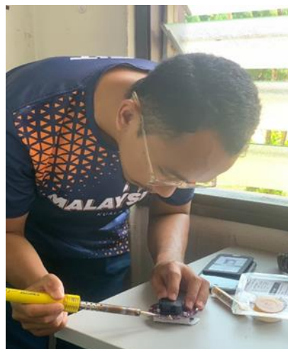
Figure 3.2 : Assembling wireless smoke sensor components
