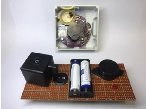
Figure 3.7 : Wireless smoke sensor with Fire alarm panel
