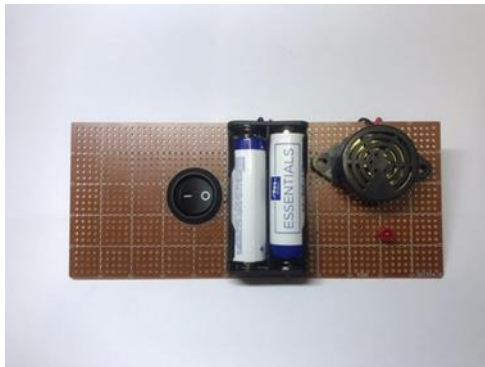
Figure 3.4 : Fire alarm panel prototype
