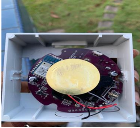
Figure 3.3 : Microcontroller integrated wireless smoke sensor
