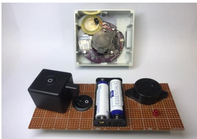
Figure 4.1 : Final Product of Wireless smoke sensor with Fire alarm panel
