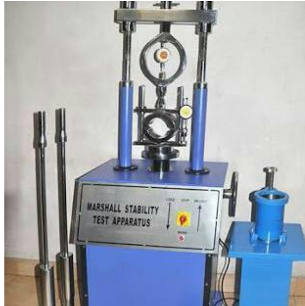
Rajah 3.3 : Marshall Stability Test
