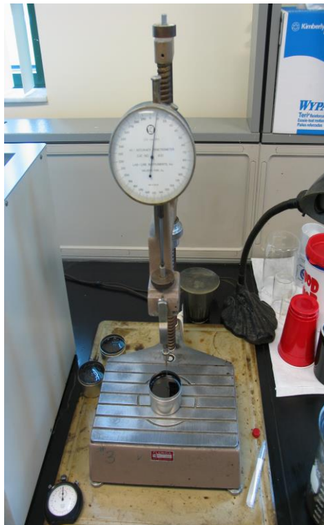
Rajah 3.1 : Penetration Test
