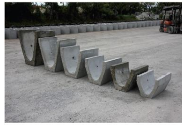
V SHAPE BLOCK DRAIN (JKR)
