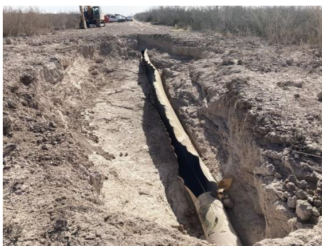
Figure 1.1.1 Pipe ruptures due to acidity in soil.
