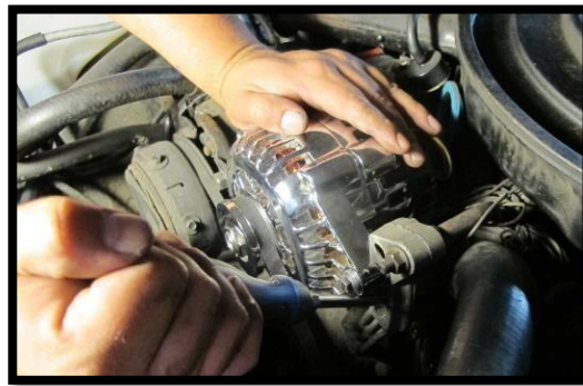
Figure 4.1 : Disassemble process for alternator
