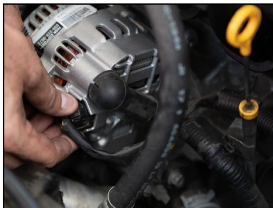
Figure 4.10 : Alternator is installed on the car
