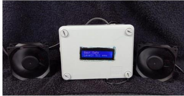
GAS LEAK DETECTOR WITH AUTOMATI AIR EXHAUST AND NOTIFIATION VIA TELEGRAM
